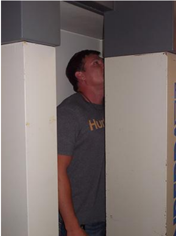
Whole body counters don't detect alpha contamination
