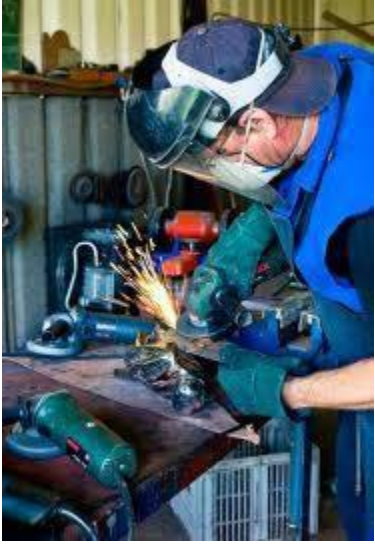
Grinding can disturb oxide layers
