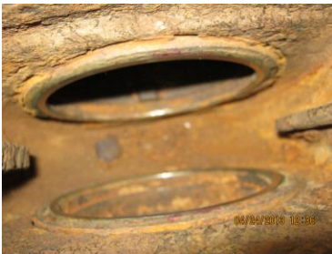
Oxide buildup on old component
